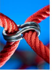
Corocord 'S' clamps are used as universal connections in Corocord products. 8mm stainless steel rods with rounded edges are pressed around the ropes with a special hydraulic press, making them the ideal connector: safe, durable and vandalism-proof, all while allowing the typical movement of rope play structures.
