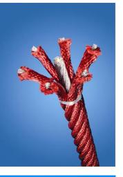
Corocord ropes with 19mm diameter or more are special 'Hercules' - type with galvanized six-stranded steel wires. Each strand is tightly wrapped with PES yarn, which is melted onto each individual strand. The ropes are highly wear-and vandalism-resistant and can be replaced at site if needed.
