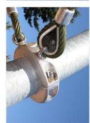
Corocord alum inium clamps are used as connectors between steel posts and rope. Two alum inium castings are bolted together. The height of the clamps is thus variable.
