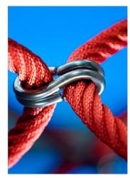
Teter or more areCorocord 'S' clamps are used as universal<br/>connections in Corocord products. 8mm<br/>stainless steel rods with rounded edges are<br/>s melted ontos melted ontopressed around the ropes with a special<br/>hydraulic press, making them the ideal<br/>connector: safe, durable and vandalism-proof,<br/>all while allowing the typical movement of rope
