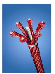
Corocord ropes with 19mm diameter or more are special 'Hercules' - type with galvanized sixstranded steel wires. Each strand is tightly wrapped with PES yarn, which is melted onto each individual strand. The ropes are highly wear-and vandalism-resistant and can be replaced at site if needed.
