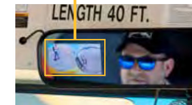
The Full View Camera System displays the most appropriate view based on the situation at hand, including backing up, opening the door, or the view of the front, side or rear of the bus.
